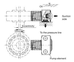
oil to the clamping devices for tools and machine components (tailstock, columns, table, spindle box) or to the jigs used for clamping work; laboratory-type table presses for compression and tensile test samples; e.g. pump element driven via a hand lever, etc.
