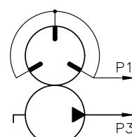
Radial piston pump - Radial piston pump
