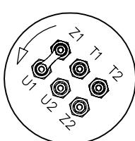
The terminals U1, U2, Z1(Z2), and PE are accessible as described under ① ... ④ above for the 3-phase mains version. The motor is internally connected ex-works, like described in sect 3.3. An alternation is neither required nor possible.
