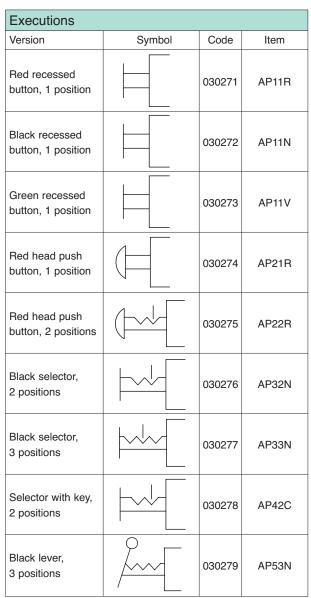
The head push button 2 positions type AP22R can only be used with the valves normally open.
