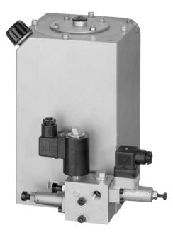
Type 3 HK44/1-H4,2 - B31T/200-EM11V-12/5-WG230 Version for max. flow of 20 lpm and permissible pressure of 450 bar, intended for single acting consumers, see sect. 2.3
