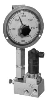
Type 1 MP44-H7,0/B10 - **B1/300-1-31D-G24** Version for a max. return flow to the tank of 6, 12, or 25 lpm and permissible pressure of 500 or 700 bar intended for single acting consumers, see sect. 2.1
