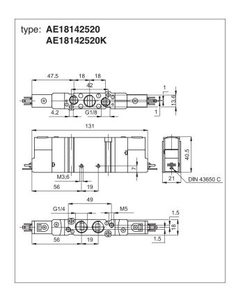
Series of spool valves with reduced dimensions and low electrical consumption, thanks to which they can be operated directly by electronic systems.
