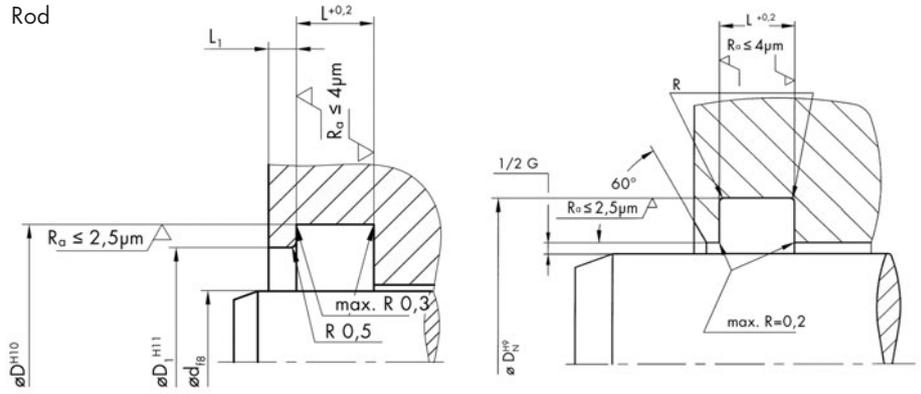
The radius R in the wiper designs AE 40 and AE 42 is dependant on the height of the wiper, as follows:
