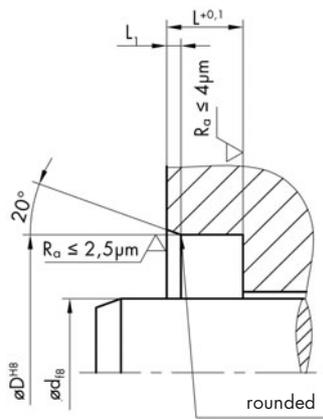
These wipers are easily installed in axially accessible housings provided the lead-in chamfer L is in accordance with the following table:
