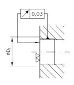
Counter sinking D<sub>1</sub> = D + 0.5 ... 1 mm
