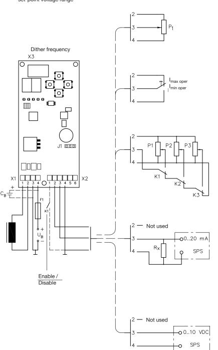
**Example a:** Operation with an external setpoint value potentiometer
