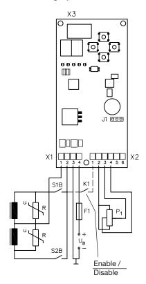
This mode of operation requires a remote-control potentiometer for central tapping and side recognition of two positively connected direct. switches SB 1 and SB 2 for solenoid coils 1 and 2
