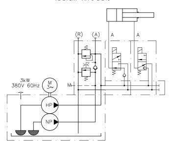
The use of a NE 70 in in a hydraulic die clamp
