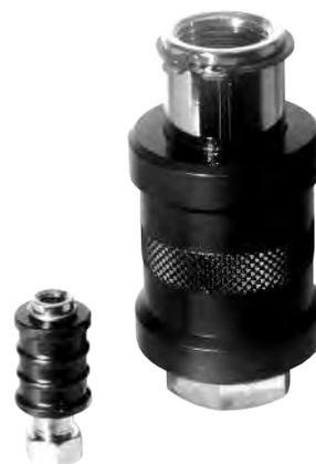
Series of slide valves manually operated. In line mounting they work to close the supply and at the same time exhaust the downstream circuit air.
