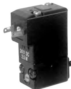
Series of directly operated poppet valves for single or manifold sub-bases, standard with coil and without connector. The single base is M5 threaded. The manifold bases can be supplied with M5 ports or with integral 4 mm push-in fitting. For sub-bases see page 2.2.2. For the connectors type A19207.. see page 2.210.10.
