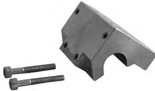
Series of plates for the direct assembly of the valves A1 to the tube (or tie-rods) of the cylinder AMA / AMT / CM. These plates have multiple mounting holes for at least two sizes of A1 valves (depending on cylinders bore).
