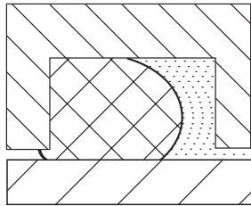
Back-up rings are used to prevent O-rings from gap extrusion. In the case of the combination of rising pressures and large sealing gaps there is the risk, that the O-ring material will be pressed into the sealing gap on the low pressure side. If this is repeated several times and the pressure continues rising, the O-ring can be damaged irreversible and finally get completely destroyed.
