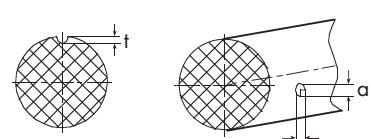
**Ideally**, the inner diameter ( $\varnothing d_1$ ) is measured by using conical with step barrel gauges. The individual barrel gauges are designed to suit each particular measuring range. A circumferential measuring tape is sufficient for O-rings with an inner diameter of more than 250 mm. Non-contact optical measuring is advised for very small O-rings (less than 1 mm inner diameter).
