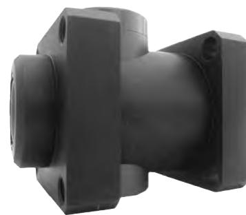
Series of locking rod units for cylinders DIN ISO 6431 and VDMA 24562 with pneumatic releasing and rod mechanical locking obtained through a double jaw (the locking is pneumatic in the type normally open).
